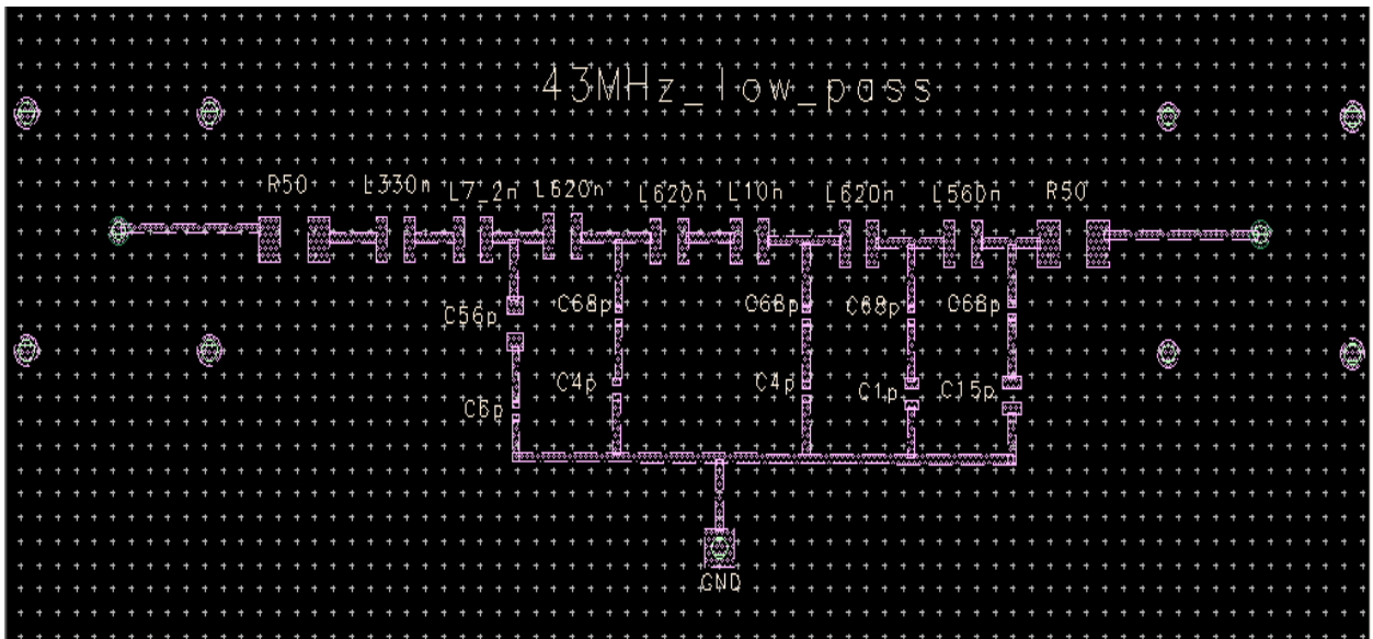
Figure 8: Layout of 43MHz low pass filter
